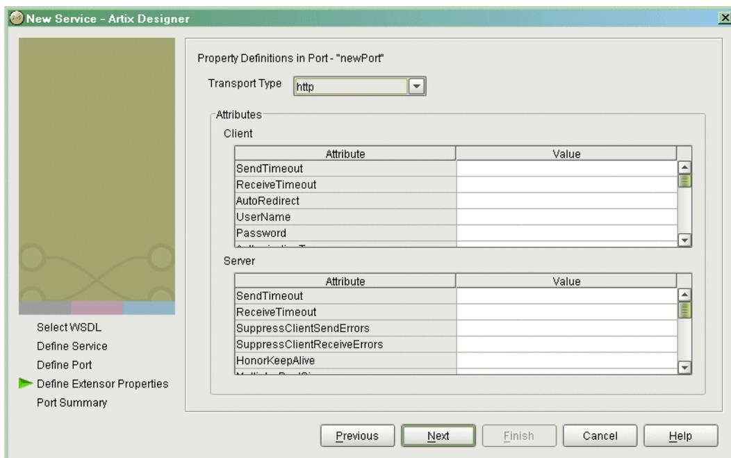
**Figure 23:** Selecting an HTTP Transport Type
