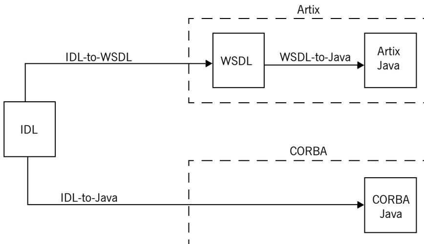
**Figure 1:** *Artix and CORBA Alternatives for IDL to Java Mapping*
