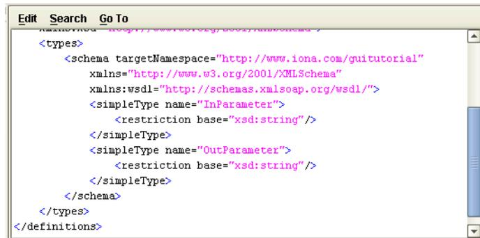
A screenshot of a software application window titled "Edit Search Go To". The window displays XML code for a WSDL file. The code includes a schema definition with two simple types: "InParameter" and "OutParameter", both restricted to the base type "xsd:string". The code is as follows:
