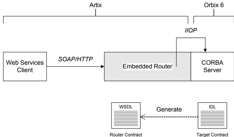
**Figure 1:** Artix Router Embedded in a CORBA Server
