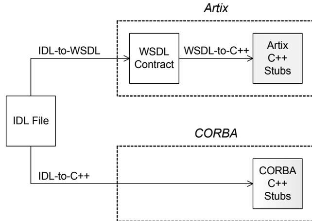
**Figure 1:** *Artix and CORBA Alternatives for IDL to C++ Mapping*
