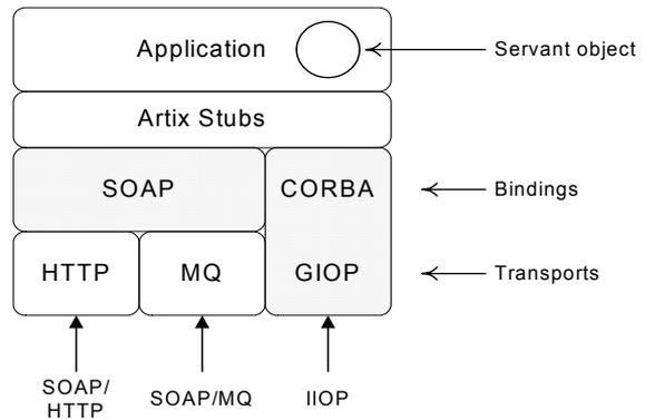
**Figure 1:** *Artix Application with Multiple Bindings and Transports*
