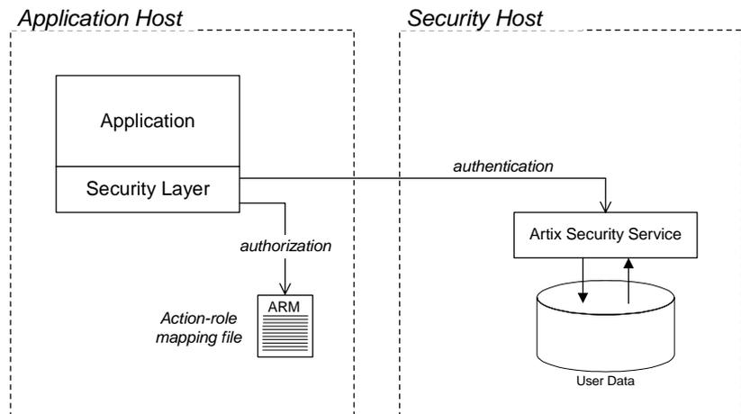
**Figure 25:** Locally Deployed Action-Role Mapping ACL File
