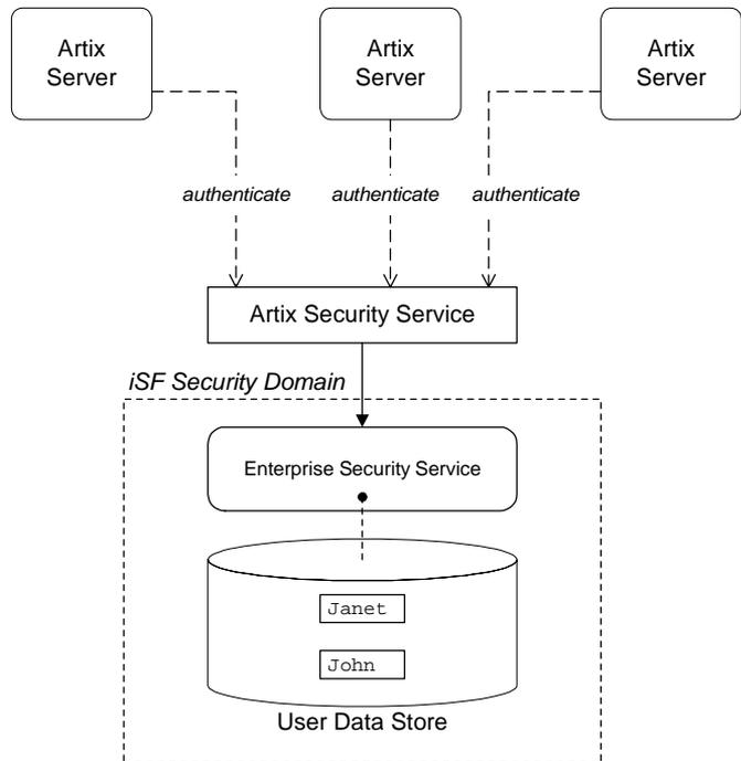
**Figure 21:** Architecture of an Artix security domain
