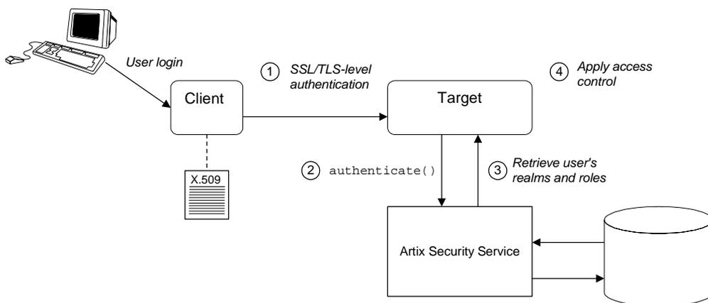
**Figure 10:** Overview of Certificate-Based Authentication with HTTPS
