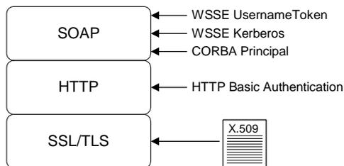
**Figure 6:** *Protocol Layers in a SOAP Binding*
