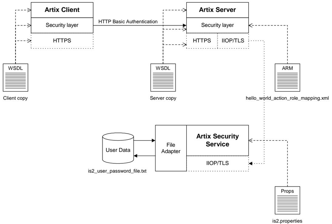
**Figure 4:** *The Security Layer in the HelloWorld Example*
