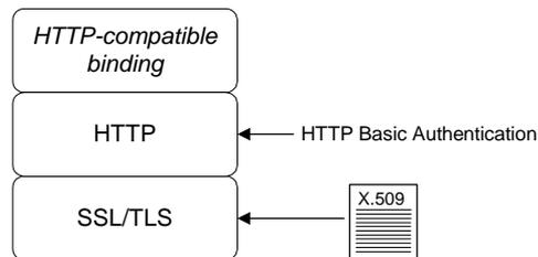
**Figure 5:** *Protocol Layers in a HTTP-Compatible Binding*
