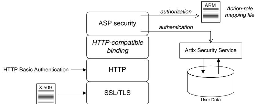
**Figure 9:** *HTTP-Compatible Binding Security Layers*
