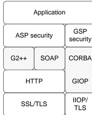
**Figure 8:** Example of an Application with Multiple Bindings
