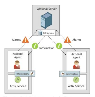
Figure 1: Artix—Actional Integration Architecture
