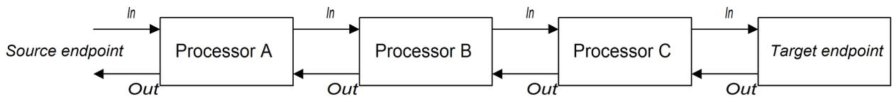
Because each processor processes the *In* message *before* delegating the exchange to the next node, the *In* message gets processed in the order shown in [Figure 3 on page 29](#) (left to right). In addition, because each processor process the *Out* message after delegating the exchange to the next node, the *Out* message gets processed in the reverse order (right to left).
