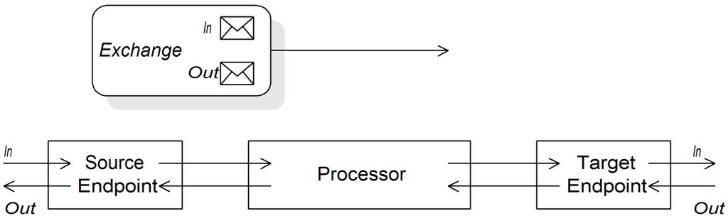
Figure 1 on page 16 shows an exchange object passing through a route. In the context of a route, an exchange object gets passed as the argument of the `Processor.process()` method, which means that the exchange object is directly accessible to the source endpoint, the target endpoint, and all of the processors in between.
