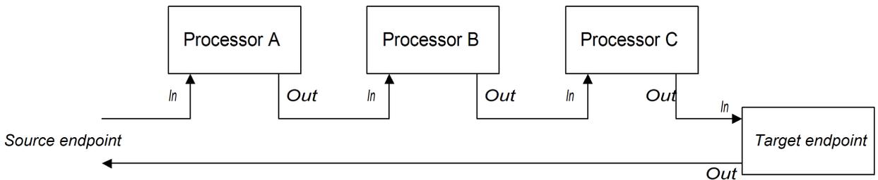
The processors in the pipeline look like services, where the *In* message is analogous to a request and the *Out* message is analogous to a reply. In fact, in a realistic pipeline, the nodes in the pipeline are often implemented by Web service endpoints (for example, using the CXF component).
