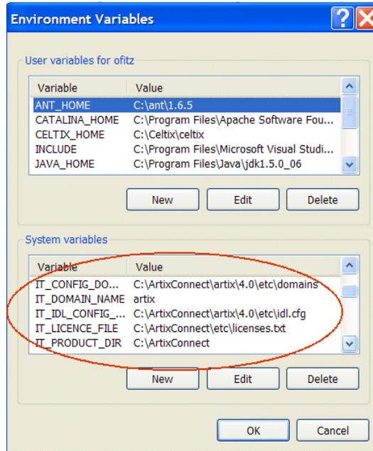
**Figure 2:** *Setting Environment Variables Manually*
