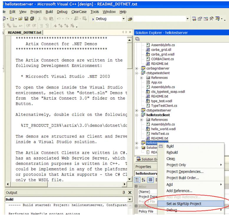
**Figure 7:** Running the Hello World Server—Set as StartUp Project
