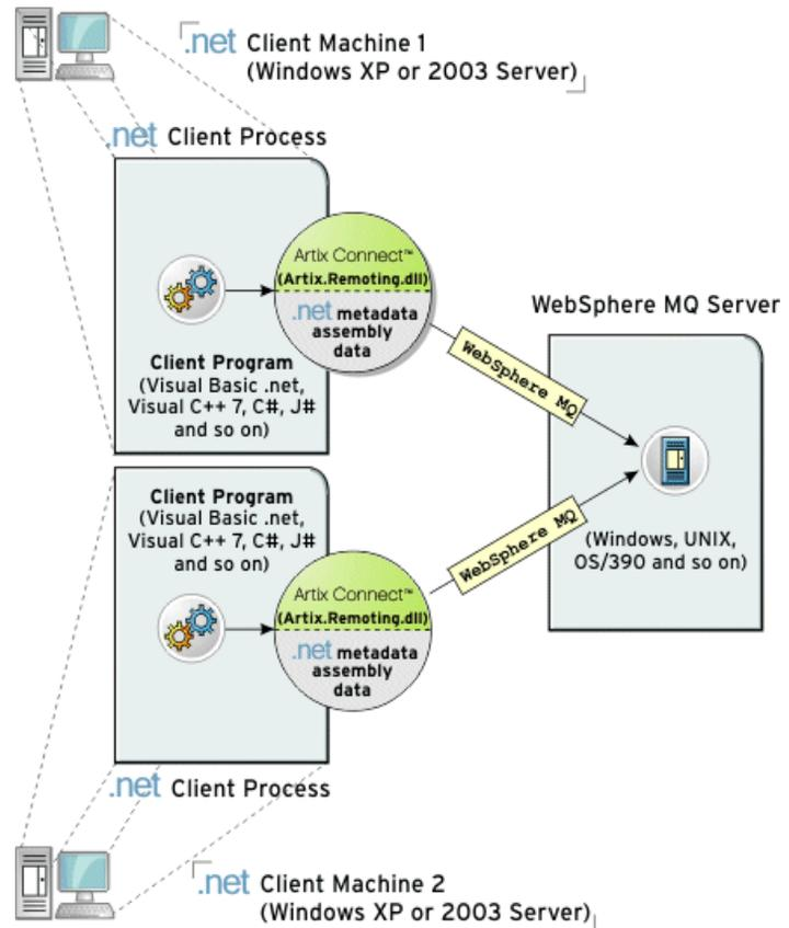
Figure 25: Typical Deployment Scenario
