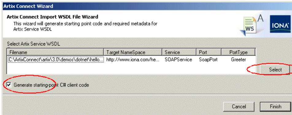
**Figure 16:** *Selecting WSDL File Using Artix Connect Wizard*
