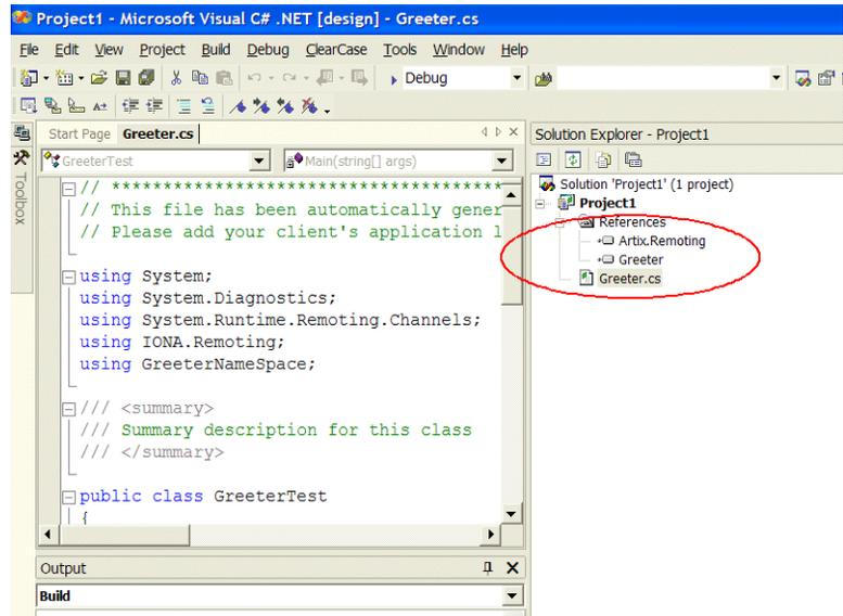
**Figure 17:** Required Files Added to Project by Artix Connect Wizard
