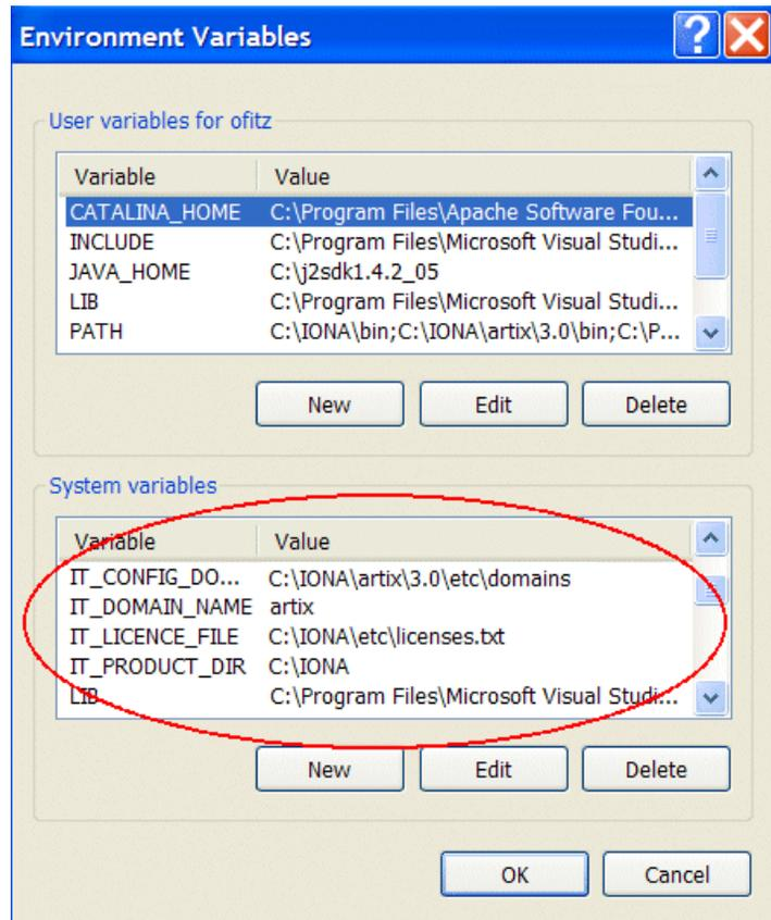
**Figure 27:** *Setting Environment Variables Manually*
