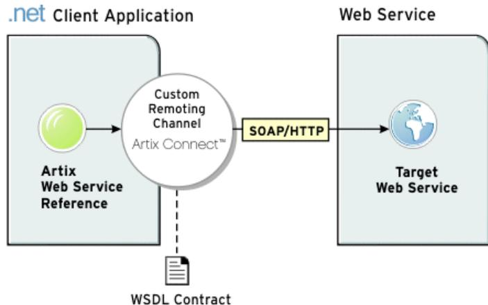
**Figure 2:** .NET client invoking on SOAP over HTTP Web Service
