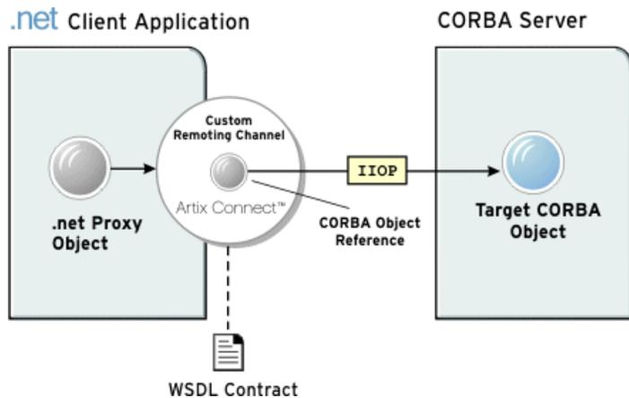
**Figure 3:** .NET client invoking on a CORBA server over IIOP
