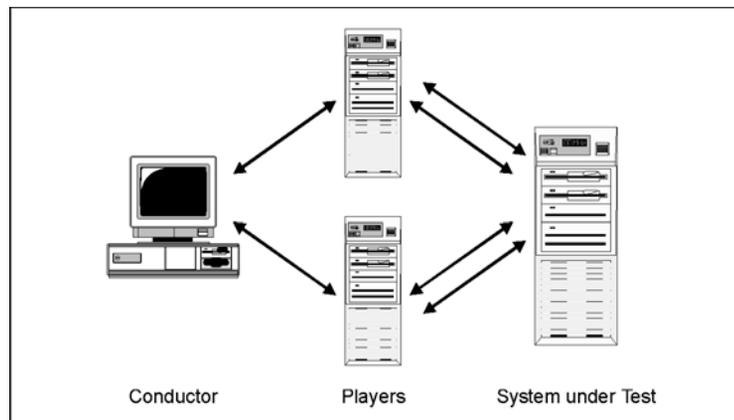
**Figure 1-1.** Test Components
