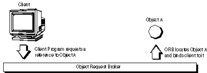
Figure 2.1 Client program acting on an object
