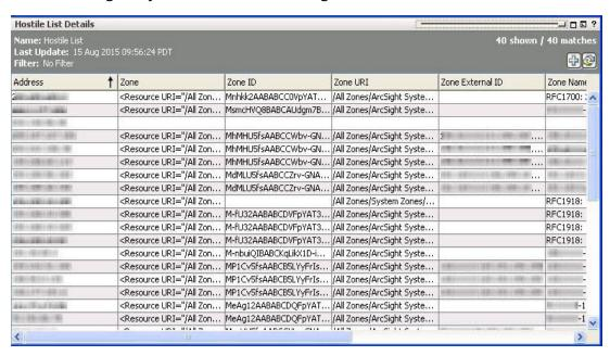
Entries written to an active list can be read by other rules, data monitors, reports, and threat evaluation processes. If you find that you use active lists heavily and the memory you have allocated for a particular active list is insufficient, you can adjust its size limit using the Active List Editor. Heavy active list usage can affect overall system performance.
