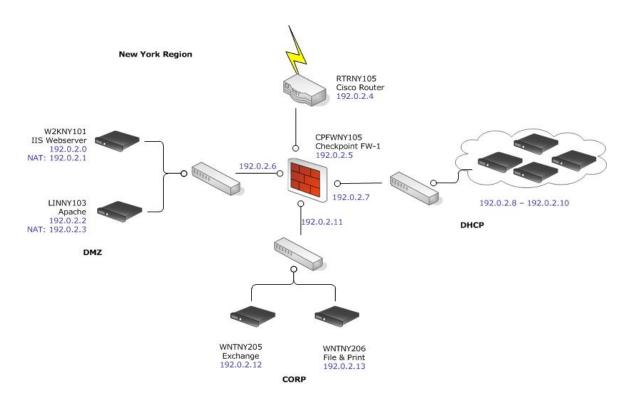
The portion of the example enterprise shown above contains web servers in a DMZ, e-mail and file-and-print servers, and a range of desktop PCs that sit behind a firewall. All traffic is directed by a Cisco router.
