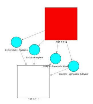
This graph shows the events that indicate a successful backdoor asylum attack on an ISS web server. In the ArcSight Console, you can double-click any node to investigate its origin.
