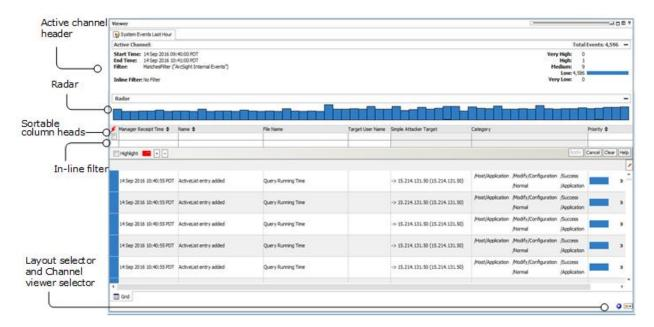
Each line item in the active channel view represents an event. The flash icon ( ) in the first column indicates a correlation event generated by a rule being triggered. Right-click any line item for an array of investigative tools. Double-click any item to view its details in the Inspect/Edit panel.
