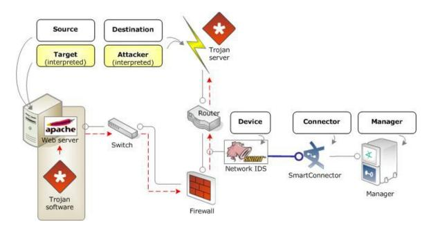
In a Trojan attack, the source is one of your own network assets, but the attacker is considered to be the outside entity that installed the Trojan software.
