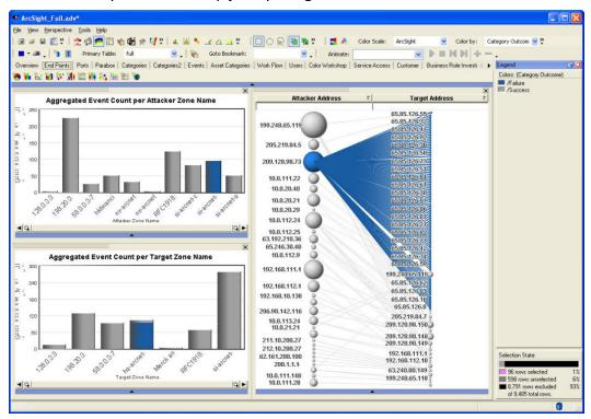
Using Interactive Discovery's visual selection tools, you can easily find and investigate potential attacks. This example shows an attacker with failed connections to many targets, which could indicate a port scan or worm.
