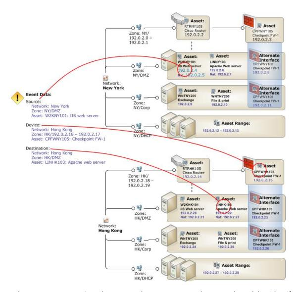
When an event comes into the system, the Manager uses the network model to identify the assets involved in the event. In this example, the endpoints involved in the event are circled in red.
