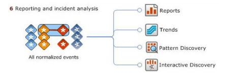
ESM batch tools work on processed events to produce reports, discover new patterns, and analyze output data using interactive graphics.
