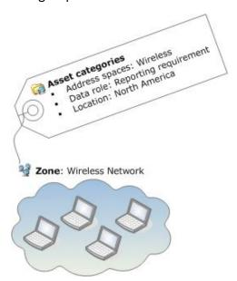
For situations where assets are not fixed, such as a wireless or VPN network, you can assign categories to a zone. For example, if a zone is categorized as confidential, you can write a rule that detects any unencrypted traffic crossing that zone, which can trigger the firewall to drop the connection or to notify an investigator.
