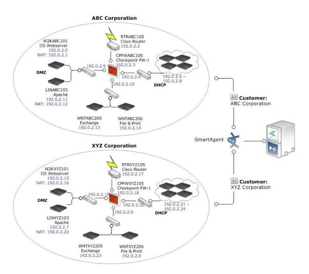
The Customer designation is usually used in an Managed Security Services Provider situation to track assets that belong to a cost center. If you do not have outside customers or an internal system of cost centers to track, you do not need to create Customers.
