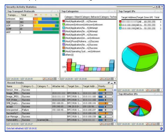
The Security Activity Statistics dashboard is just one of the standard dashboards that displays a variety of system status data monitors, which communicate the overall state of your network security. Dashboards can also display query viewers.
