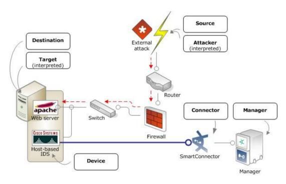
The source of an event that involves two network assets can also be an attacker if a network analyzer interprets the event as hostile. In a typical external attack, the destination (or target, if applicable) is one of the assets on your network. The attack represented here was detected and reported to ESM by a host-based IDS system.
