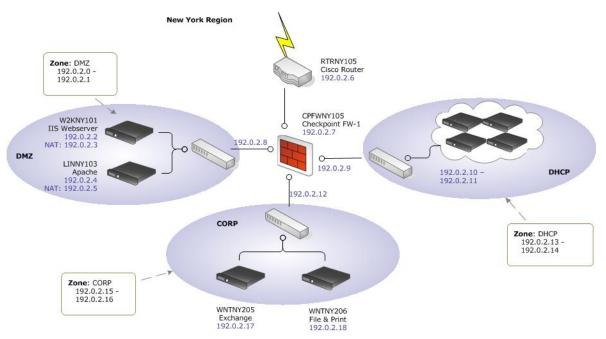
Each endpoint represented in a given event, for example the source, destination, SmartConnector, device, and so on, has a zone, or network subnet, associated with it. Zones
