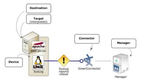
Routine network activity involving only one network asset, such as a SysLog reporting a system reboot, have only a destination and target and no source and attacker.
