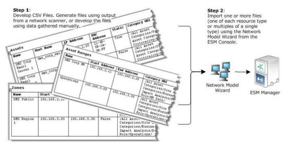
Create a CSV file for each type of asset resource you want to create, then run the Network Model wizard to import it into the Manager. In a production setting, you would likely run a report from a network scanner and edit the output to match the format required by the Network Model Wizard.
