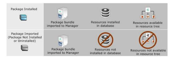
A package that has been *installed* loads its resources into the database and makes them accessible in the Navigator panel resource tree. The package icon in the Navigator panel package view will appear blue.
