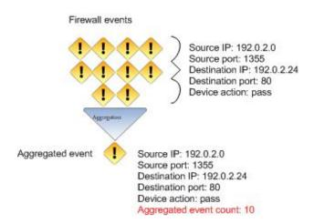
If the 30-second time frame expires and the connector has received only two matching events, the connector will create a single aggregated event with an aggregated event count of two. If 900 matching events come in during the 30 seconds, the connector would create 90 aggregated events, each with an aggregated event count of 10.
