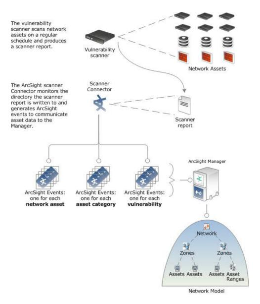
Vulnerability scans report network model and vulnerability data, which is read by a scanner SmartConnector and communicated to the Manager in a series of events. Vulnerability scans can be used to populate and update the baseline network model.
