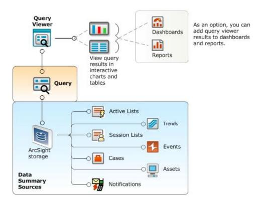
Query viewers combine the SQL querying ability of trends and reports with the drill-down capabilities of active channels in a single resource. The flexibility of SQL queries with access to drill-down details enables you to track how a situation is developing in real time. Querying the focused data set of a trend table is more performance friendly than creating low-level active channels.
