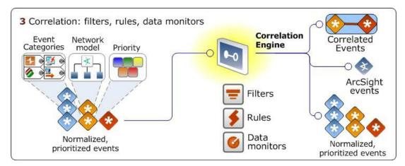
Events that have been tagged with event categories, priority evaluations, and network model information are then processed by the correlation engine, where filters, rules, and data monitors connect the dots, find the events of interest, and can initiate immediate response.
