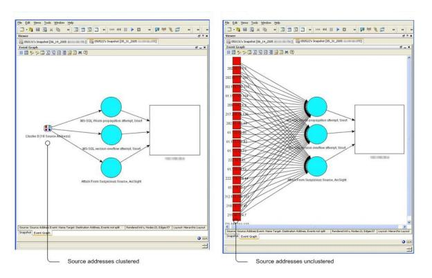
Toggle between multiple views in the Snapshot window using tabs. Unclustering the source address nodes allows you to see the details of those nodes.
