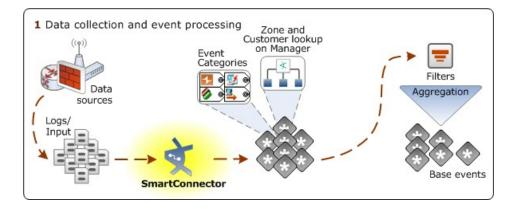
A data source on a network node generates events, which are collected by an ArcSight SmartConnector. The connector normalizes the data into the ESM schema, then tags it with event categories and looks up zone and customer attributes from the ESM network model. You can also configure the SmartConnector to filter and aggregate events to reduce the volume of the event stream.
