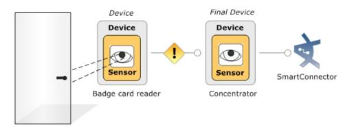
A sensor is the component of a device that actually detects the activity. Devices can report to a SmartConnector through a chain of multiple devices.
