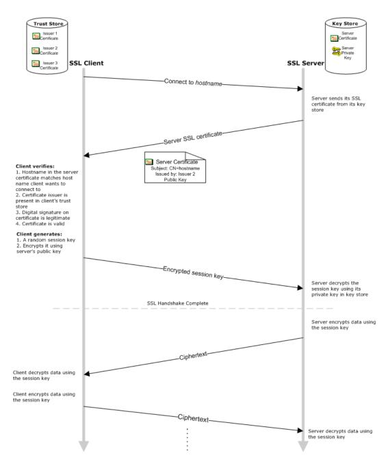
With client-side authentication, the server requests the client's certificate when it sends its certificate to the client. The client sends its certificate along with the encrypted session key.
