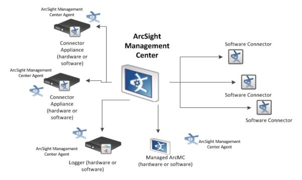
ArcSight Management Center uses the concept of nodes to manage various entities. A node is a networked ArcSight product that can be centrally managed using ArcSight Management Center. Each node is associated with a single networked host that has been assigned either a hostname, an IP address, or both.
