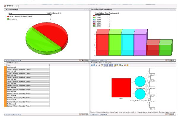
The Compliance Risk Score Overview dashboard is a centralized heads-up display that shows the current state of compliance for each of the NERC CIP Standards by displaying the results of Compliance Risk Score Overview last-state data monitor. The dashboard summarizes your environment's overall state of compliance with the NERC CIPS as determined by correlation rules triggered for each family as shown in the following figure.
