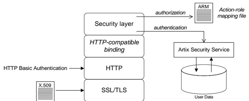
**Figure 10:** HTTP-Compatible Binding Security Layers
