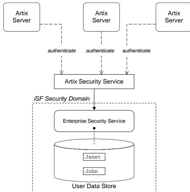
Figure 27: Architecture of an Artix security domain
