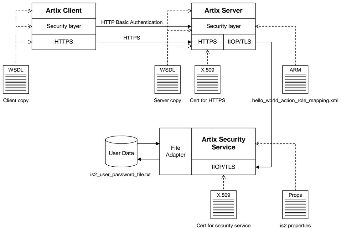
Figure 1: Overview of the Secure HelloWorld Example
