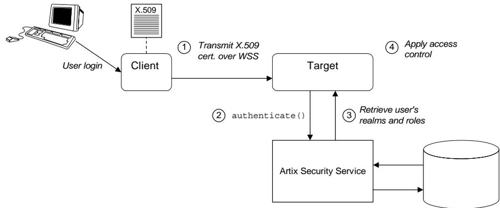
Figure 13: Overview of Certificate-Based Authentication with WSS
