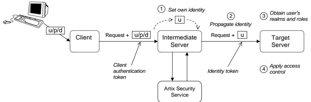
**Figure 16:** Three-Tier CORBA System Using CSIv2
