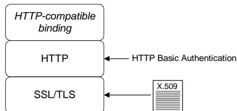
**Figure 6:** *Protocol Layers in a HTTP-Compatible Binding*
