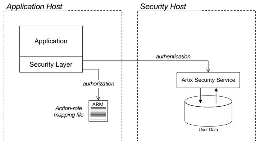
**Figure 31:** *Locally Deployed Action-Role Mapping ACL File*
