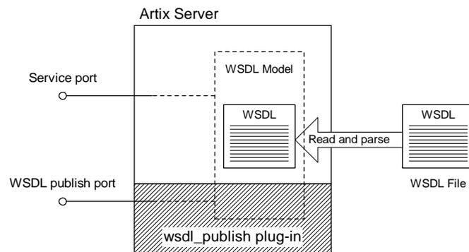
**Figure 35:** Endpoints Used by the WSDL Publishing Service
