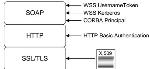
**Figure 7:** *Protocol Layers in a SOAP Binding*
