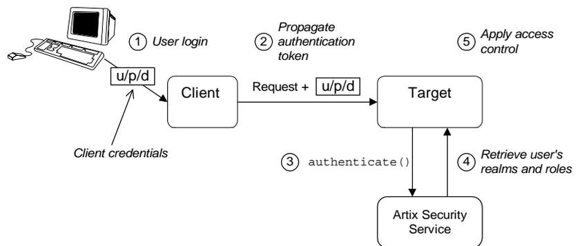
**Figure 15:** Two-Tier CORBA System Using CSI Credentials
