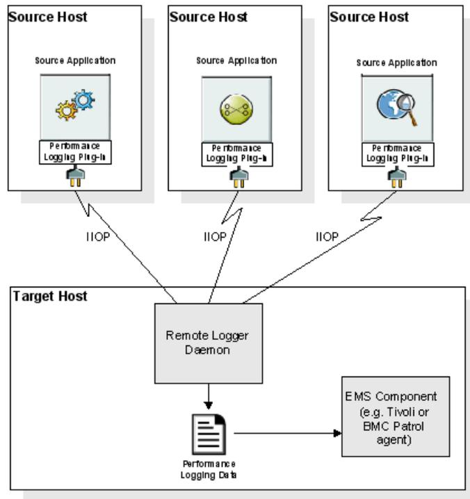
Figure 1: Remote Logging Framework
