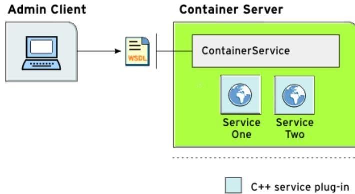
**Figure 3:** *Artix Container Architecture*
