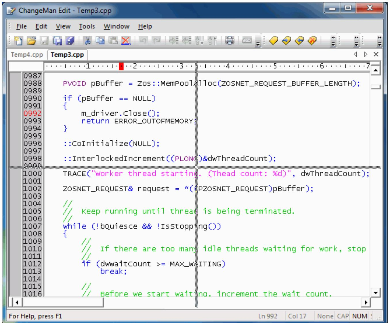
The window panes are divided by a splitter bar. You can resize the window panes by dragging the splitter bar. To remove a window pane, just move the splitter bar all the way to the edge of the window.
