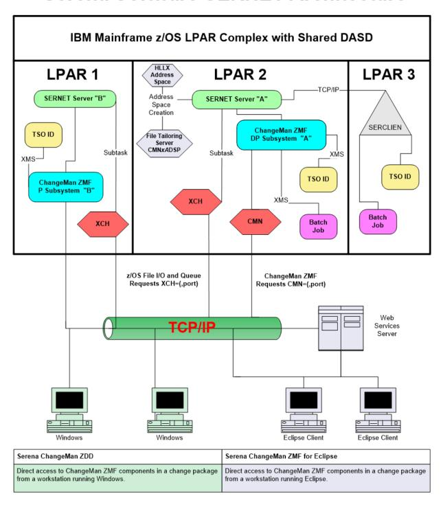
The diagram shows two Sernet instances on separate LPARs, each managing a ChangeMan ZMF instance. Users access these ChangeMan ZMF instances from the Web, from workstations in the distributed environment, and from TSO sessions in the z/OS environment. The TSO user in the last LPAR is using the Load Balancing Option of ChangeMan ZMF to work from a mainframe environment where there is no Sernet or ChangeMan ZMF instance.
