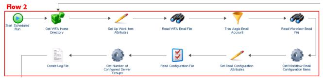
The workflow can also create multiple flows when it traverses more than one connector from an activity or when the trigger appends a new event to the work item. When there are no more active flows, execution terminates.
