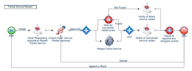
During execution, a workflow visits activities and traverses connectors in a specific order (called a **flow**). The Start of Workflow activity is the first activity the workflow executes. If the workflow contains multiple Start of Workflow activities, the workflow can have multiple simultaneous flows, as shown in the following figure.
