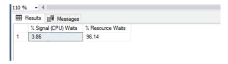
Signal waits that exceed 10-15% are typically a sign of CPU pressure.
