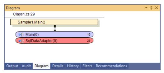
For dataflow issues, the trace starts with the first function to call the taint source, then traces the calls to the source (blue node) and ends the trace at the sink (red node). In the diagram, the source (src) and sink nodes are also labeled. A red X on a vertical axis indicates that the function called finished executing.
