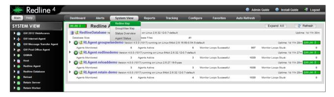
Uptime, basic vital statistics for each monitored agent, and overall percentage uptime are displayed. The Redline Agent Map is a quick and easy tool to visualize and track down outages in a system. Select the 'expand all' button to display the Redline agents which are being monitored. How the agents are displayed depends on user configuration. Agents may be organized according to alphabetical, host, redline ui, or agent Grouping
