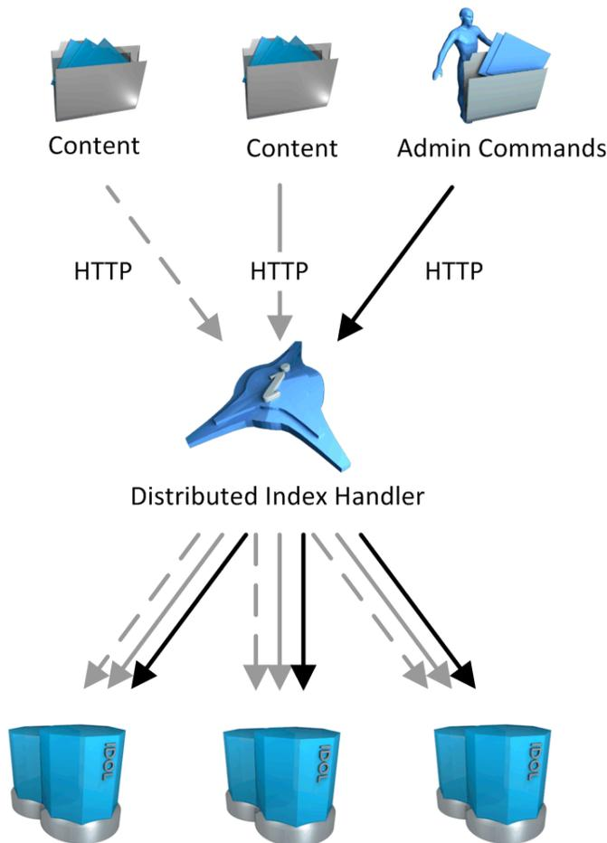
The HPE DIH sends all the index data that it receives (represented by gray arrows in the previous diagram) to all the connected IDOL Servers. The IDOL Servers are exact copies of each other, and must all have the same configuration.
