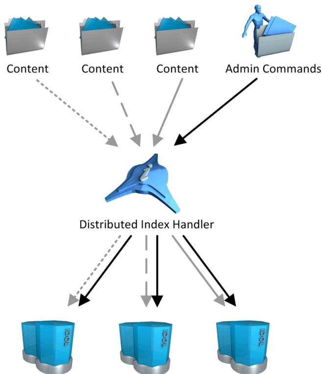
The HPE DIH distributes the index data that it receives (represented by gray arrows in the diagram above) evenly across the connected IDOL Servers. For example, if the HPE DIH connects to four IDOL servers, it indexes approximately one quarter of the data into each IDOL server. It does not split up sections of individual documents.
