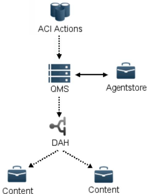
In a non-mirror mode configuration where your index is split over multiple Content components, this architecture reduces the number of additional components you need to configure. In a mirror mode configuration, you can use this architecture if you do not need to include load-balancing or failover for the QMS part of the system.
