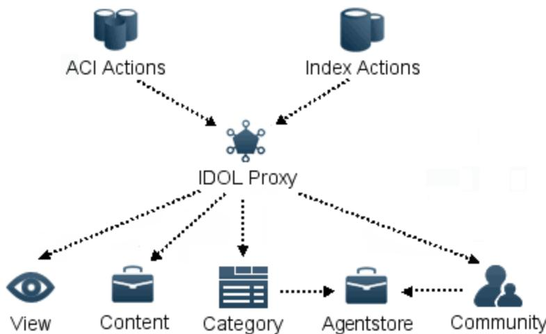
This setup is useful for training and testing, because it allows you to easily modify the configuration for the server, and you do not have to understand the whole IDOL architecture. However, for most production environments, the unified IDOL setup is too small and restrictive. For example, it has limited scalability and no failover, it is difficult to add additional Content components to increase the size of the index, and you cannot include QMS.
