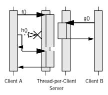
Figure 12: Thread-per-Client Server
