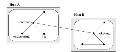
Figure 3: Naming Graph Spanning Two OrbixNames Servers
