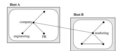
Figure 8: Naming Graph Spanning Two OrbixNames Servers
