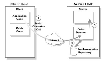
Figure 2: Automatic Launch of an Orbix Server Process
