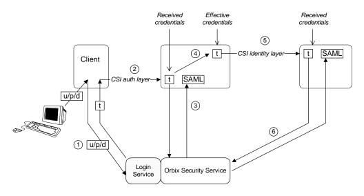
**Figure 26:** Single Sign-On Scenario without Piggybacking Roles and Realms
