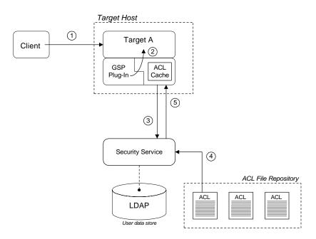
Figure 37: Centralized ACL scenario
