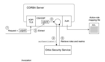
Figure 62: CSIv2 in the Orbix Security Framework
