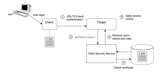
Figure 19: Overview of iSF Certificate-Based Authentication
