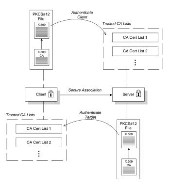
Figure 52: Target and Client Authentication
