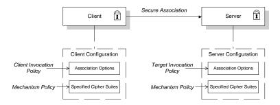
Figure 49: Configuration of a Secure Association
