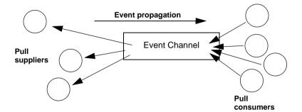
Figure 5: Pull Model Suppliers and Consumers Communicating through an Event Channel
