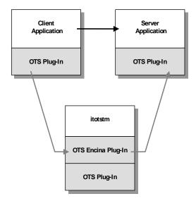
Figure 19: Using the OTS Encina plug-in with the itotstm service
