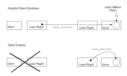
Figure 3: The Lease is Released When the Client Shuts Down
