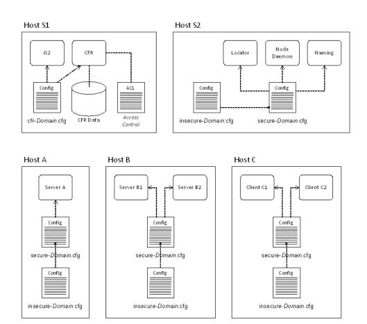
Figure 40: Overview of a Secure CFR Domain
