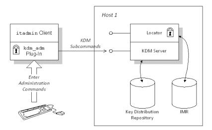
Figure 63: Using itadmin to Manage the KDM Server
