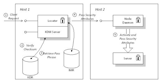
Figure 62: Automatic Activation of a Secure Server
