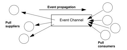
**Figure 5:** Pull Model Suppliers and Consumers Communicating through an Event Channel
