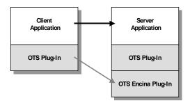
Figure 20: Loading the OTS Encina Plug-In into the Application
