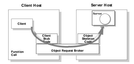
Figure 3: Invoking on a CORBA object
