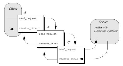
Figure 54: Client interceptors process a LOCATION\_FORWARD reply.
