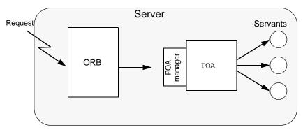
**Figure 19:** The server-side ORB conveys client requests to the POA via its manager, and the POA dispatches the request to the appropriate servant.
