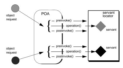
**Figure 25:** *The POA directs each object request to the servant locator, which returns a servant to the POA to process the request.*
