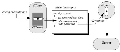
Figure 52: PICurrent facilitates transfer of thread context data to a request or reply.
