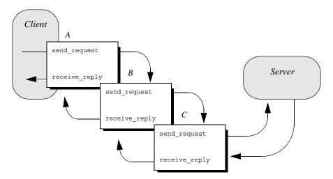
Figure 53: Client interceptors process a normal reply.
