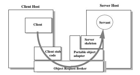
Figure 4: The portable object adapter
