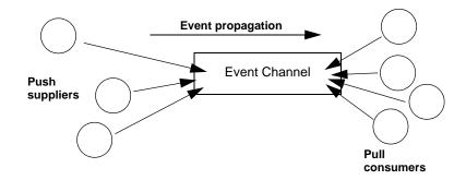
Figure 49: Push suppliers and pull consumers communicating through an event channel
