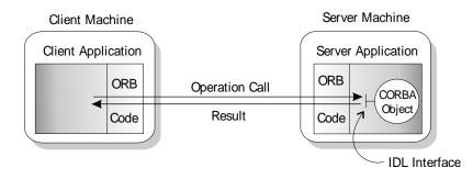
Figure 13: Client makes a single operation call on a server
