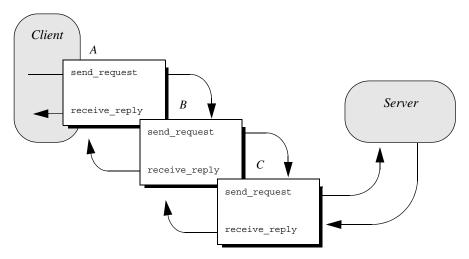
Figure 41: Client interceptors process a normal reply.
