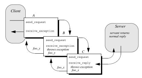
Figure 44: Client interceptors can change the nature of the reply.
