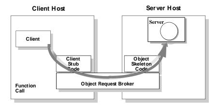
Figure 3: Invoking on a CORBA object
