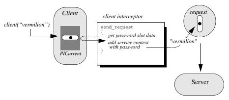
**Figure 40:** *PICurrent facilitates transfer of thread context data to a request or reply.*
