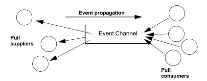
**Figure 36:** Pull Model suppliers and consumers communicating through an event channel
