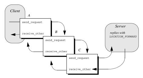
Figure 42: Client interceptors process a LOCATION\_FORWARD reply.
