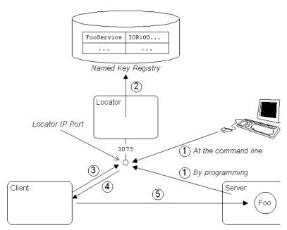
Figure 51: Using corbaloc with the Locator-Based Named Key Registry
