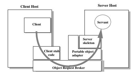
**Figure 4:** The portable object adapter
