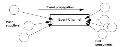
Figure 37: Push suppliers and pull consumers communicating through an event channel
