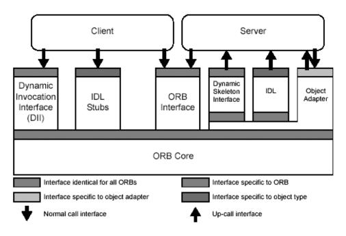
Figure 6: The Components of an ORB
