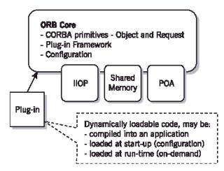
Figure 8: Orbix Plug-In Architecture
