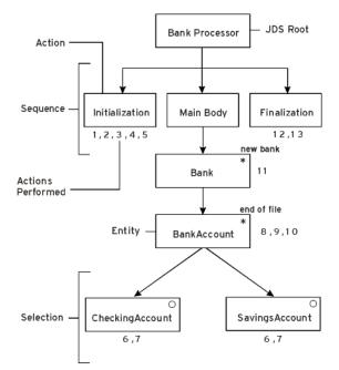
Figure 4: Jackson Structure Diagram for the Banking Application
