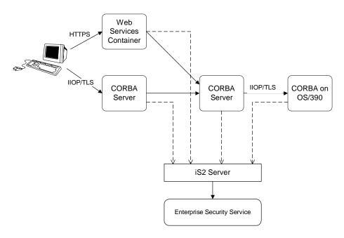
Figure 1: Example System with a Standalone Orbix Security Service
