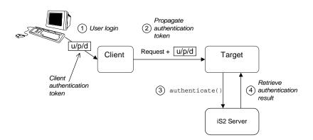
Figure 4: Two-Tier CORBA System in the iSF
