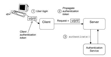
Figure 13: Basic CSIv2 Authentication over Transport Scenario
