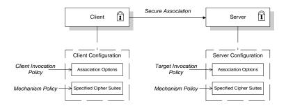
Figure 8: Configuration of a Secure Association
