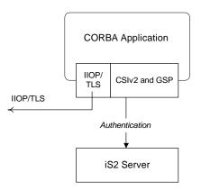
Figure 3: A Secure CORBA Application within the iSF
