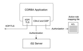
Figure 2: Security Plug-Ins in a CORBA Application
