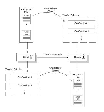
Figure 11: Target and Client Authentication
