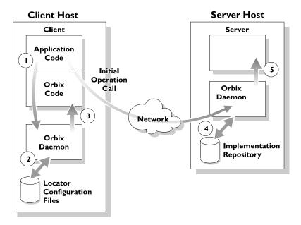
Figure 1.3: The Orbix Server Locator Mechanism
