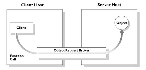
Figure 1.1: The Object Request Broker
