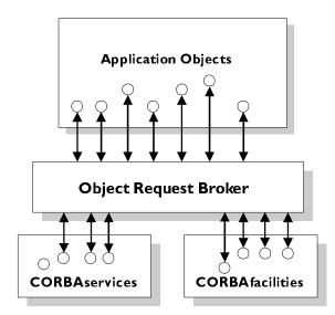
Figure 1.5: The Object Management Architecture
