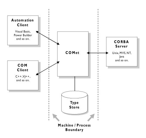
Figure 1.2: OrbixCOMet's Implementation of the Interworking Model
