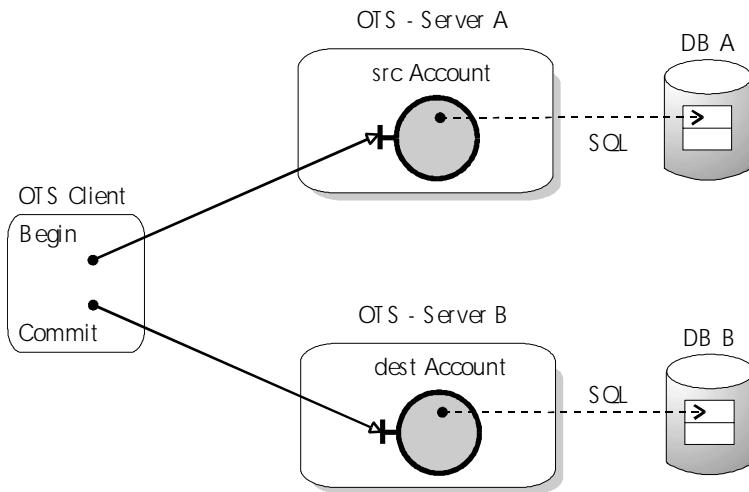
**Figure 7.3: Distributed Transaction with OTS Client.**
