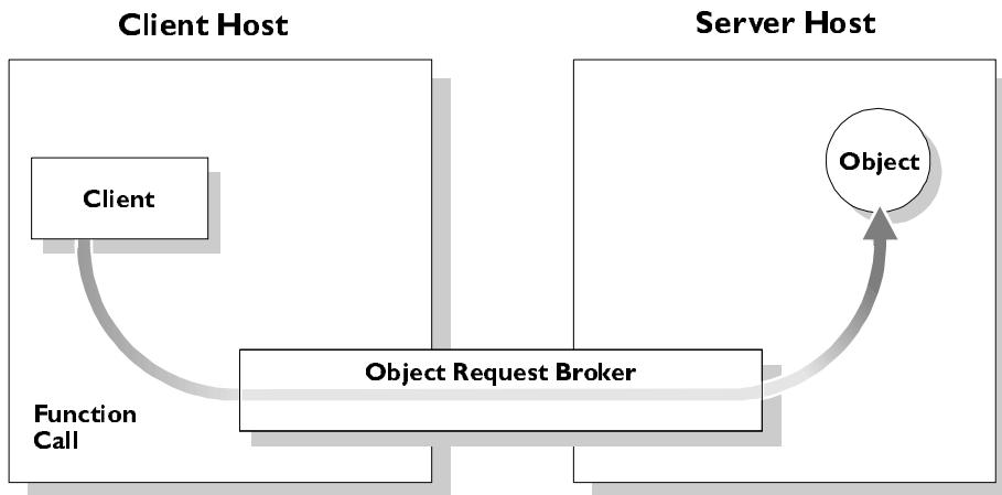
Figure I.1: The Object Request Broker
