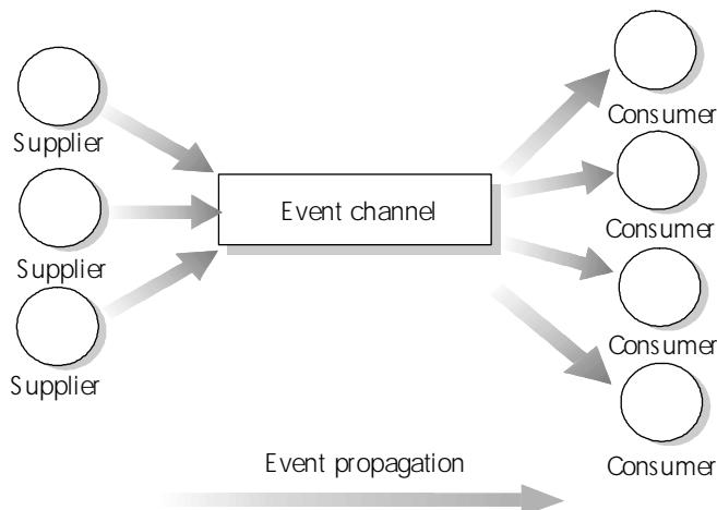
**Figure 6.1:** An Event Channel Mediates the Flow of Events from Suppliers to Consumers.
