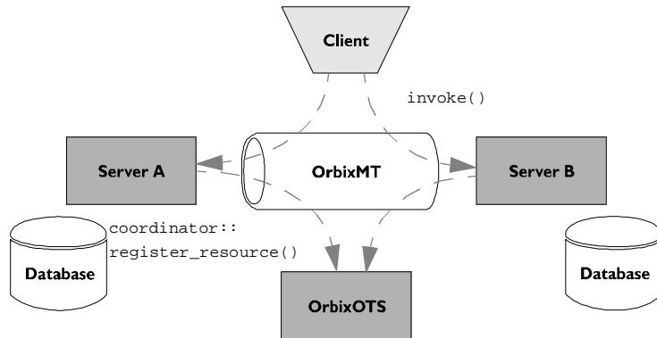
**Figure 7.7:** Server Registers with OrbixOTS when Client First Invokes
