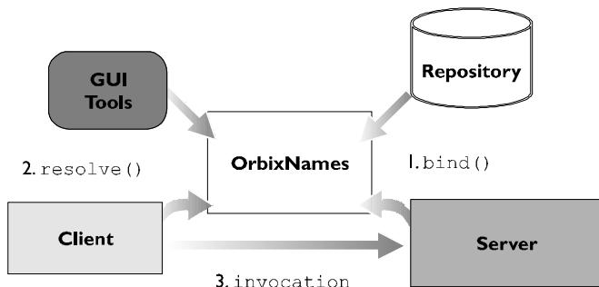
**Figure 1.7: The OrbixNames Architecture**
