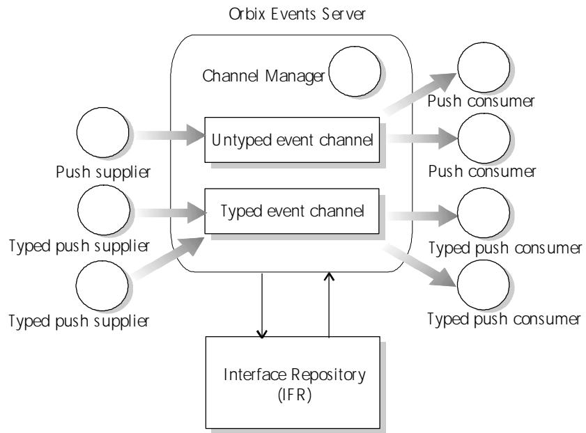
**Figure 6.3: Architecture of the OrbixEvents Server.**
