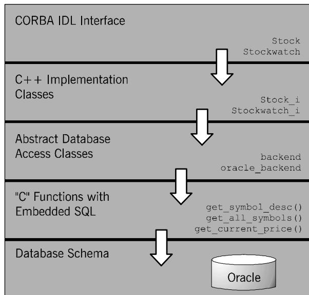
**Figure 4.4: Structure of StockWatch Server Program**
