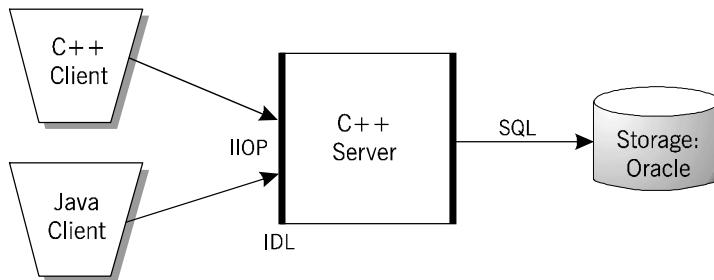
**Figure 4.3: Simple Three-Tiered Architecture**
