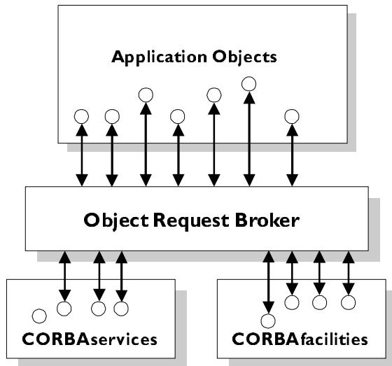
**Figure I.5: The Object Management Architecture**
