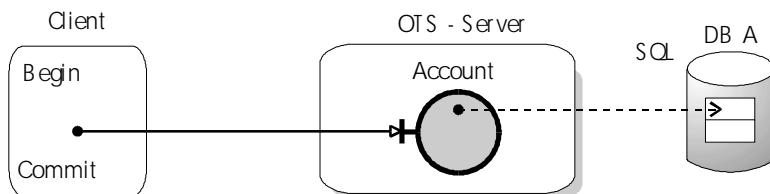
**Figure 7.5: OTS Client Invoking on a Single OTS Server.**
