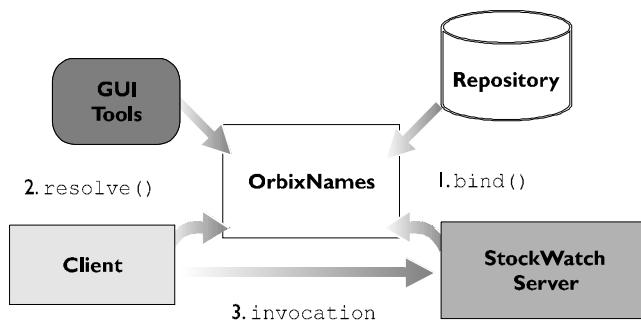
**Figure 5.1: Using OrbixNames in Orbix**
