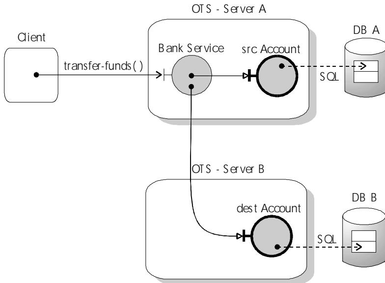
**Figure 7.4: Distributed Transaction with Ordinary Client.**
