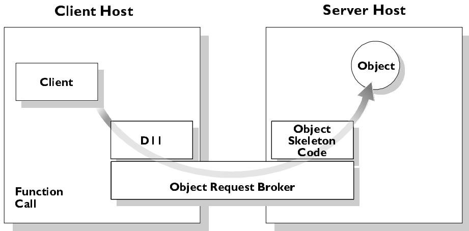
Figure 1.3: Client Invoking a Function Using the DII
