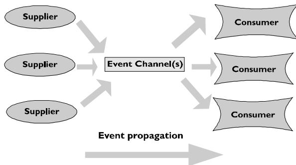
**Figure 1.8: Schematic View of OrbixEvents Architecture**
