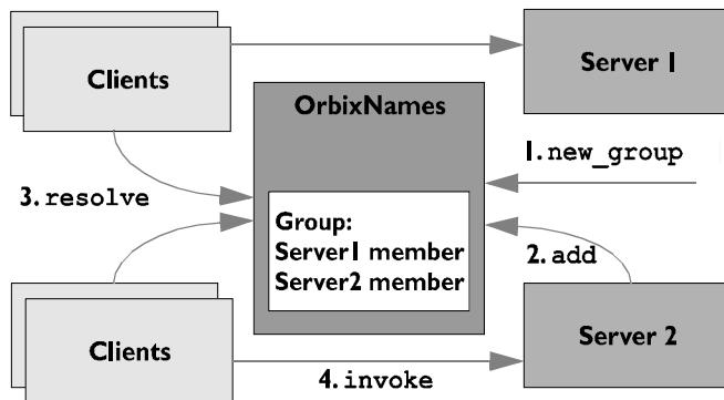
Figure 9.2: Naming Service and Load Balancing
