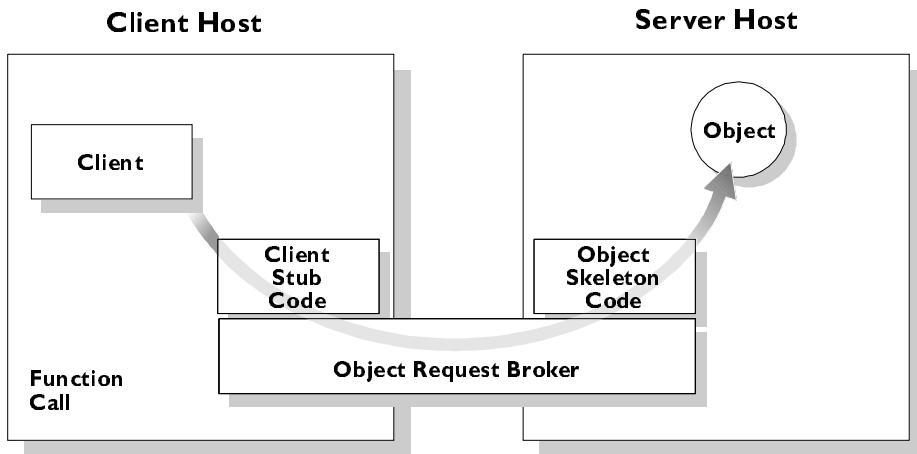
Figure 1.2: Invoking on a CORBA Object
