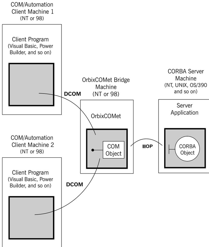
**Figure 12.5:** COM/Automation to CORBA with Bridge on Intermediary Machine
