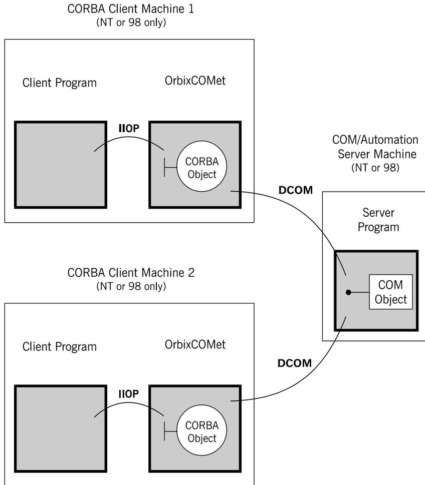
**Figure 12.2:** CORBA to COM/Automation with Bridge on Each Client Machine
