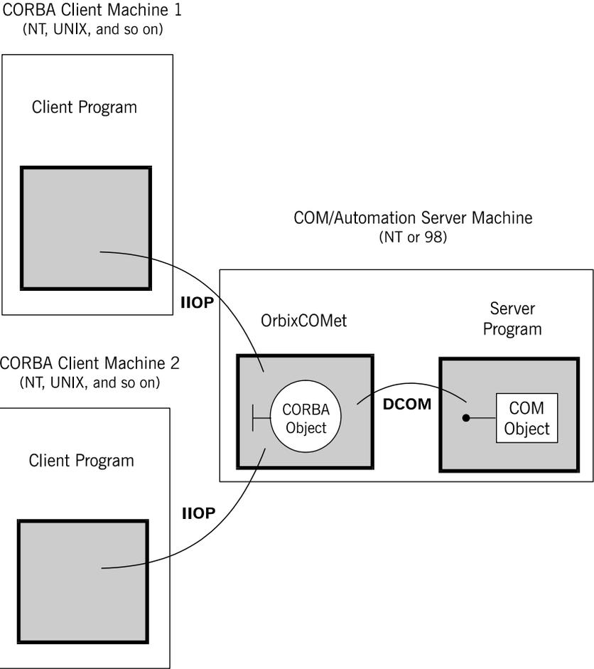
Figure 12.4: CORBA to COM/Automation with Bridge on Server Machine
