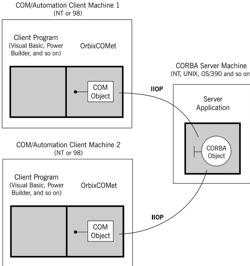
**Figure 12.1:** COM/Automation to CORBA with Bridge on Each Client Machine
