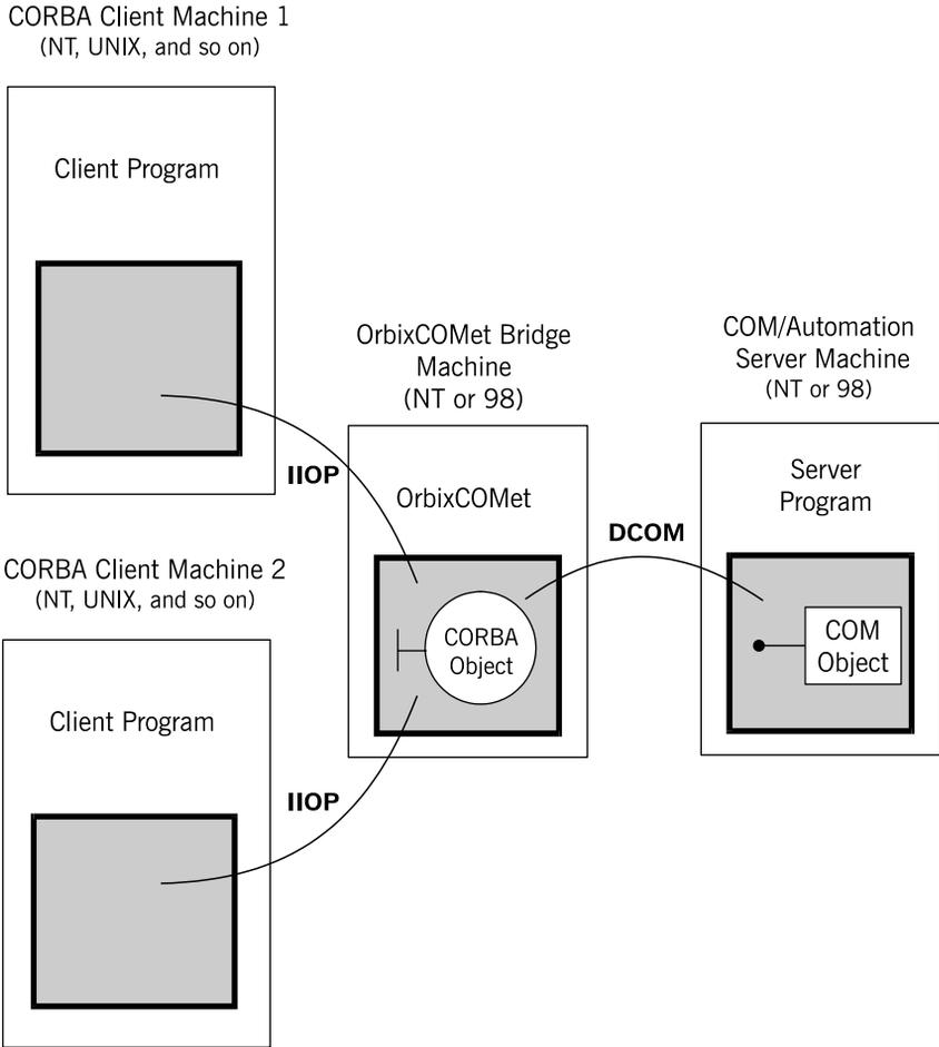
**Figure 12.6:** CORBA to COM/Automation with Bridge on Intermediary Machine
