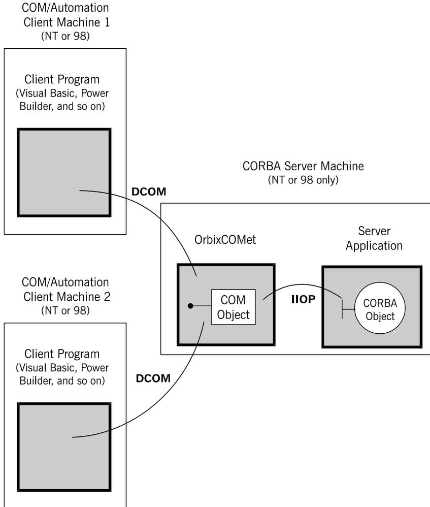
**Figure 12.3:** COM/Automation to CORBA with Bridge on Server Machine
