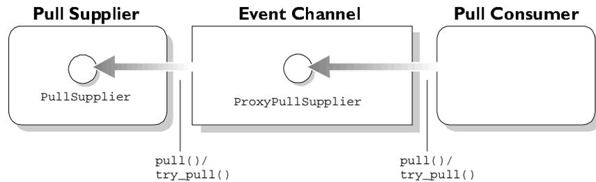
**Figure 2.4:** *Transfer of an Event Through an Event Channel to a Consumer using the Untyped Pull Model*
