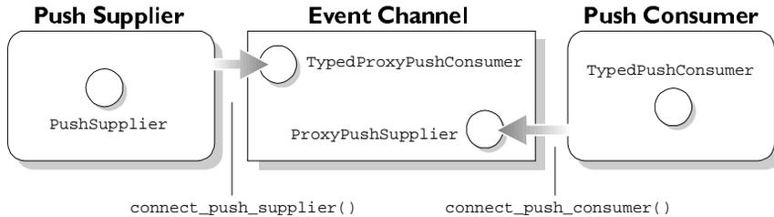
**Figure 2.5:** Push Supplier and Push Consumer Connecting to an Event Channel using the Typed Model
