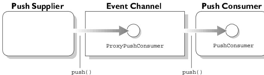
**Figure 2.3:** *Transfer of an Event Through an Event Channel to a Consumer using the Untyped Push Model*
