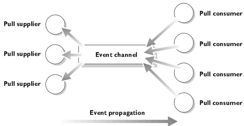
**Figure 1.5:** *Pull Model Suppliers and Consumers Communicating through an Event Channel*
