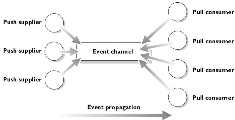
**Figure 1.6:** Push Model Suppliers and Pull Model Consumers in a Single System
