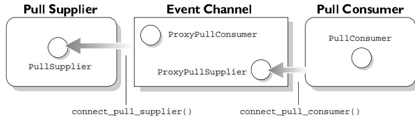
**Figure 2.2:** Pull Supplier and Pull Consumer Connecting to an Event Channel in the Untyped Model
