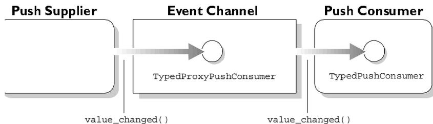
**Figure 2.6:** *Transfer of an Event Through an Event Channel to a Consumer Using the Typed Push Model*
