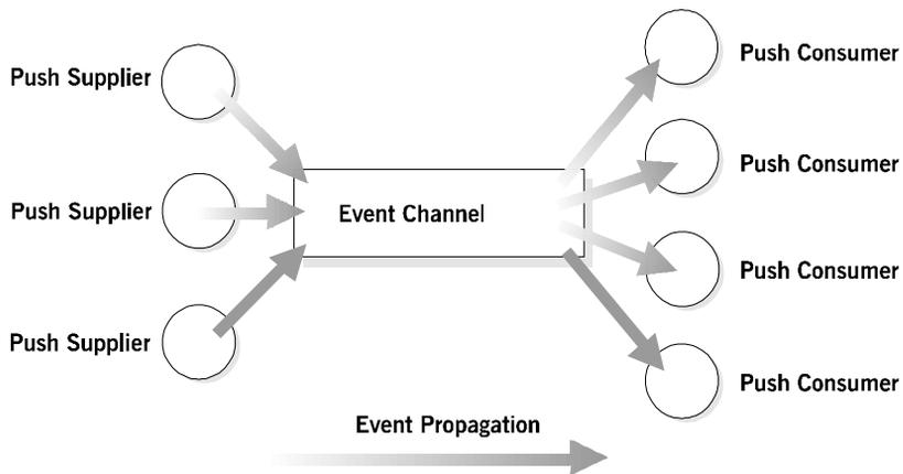
**Figure 1.4:** *Push Model Suppliers and Consumers Communicating through an Event Channel*
