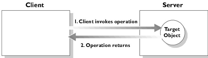
**Figure 1.1:** CORBA Model for Basic Client/Server Communications
