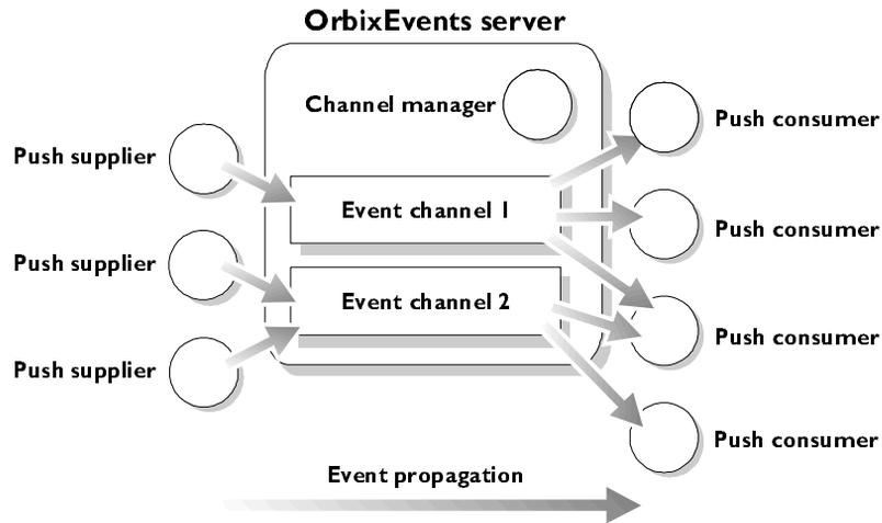
**Figure 3.1:** Example OrbixEvents Architecture with Two Event Channels
