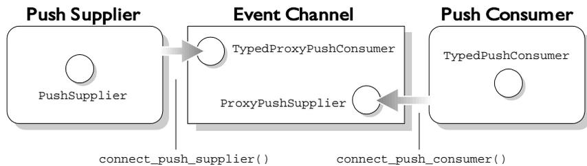
**Figure 6.4:** Push Supplier and Push Consumer Connecting to an Event Channel using the Typed Model
