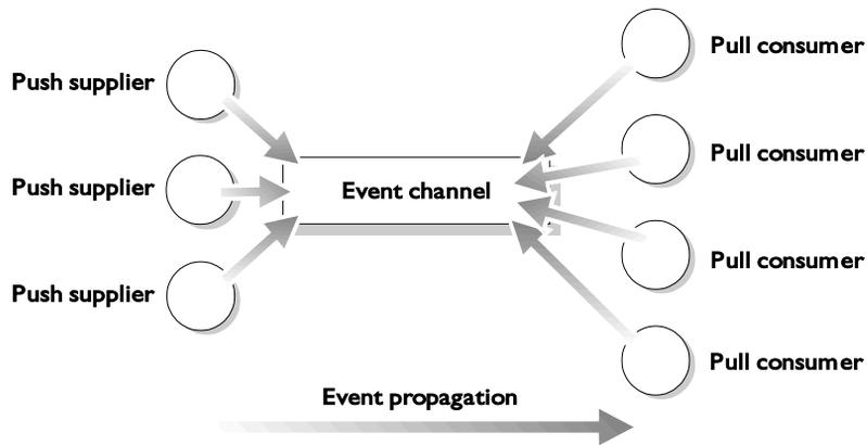
**Figure 5.6:** Push Model Suppliers and Pull Model Consumers in a Single System
