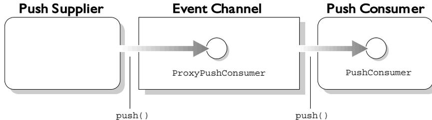
**Figure 6.2:** *Transfer of an Event through an Event Channel to a Consumer using the Untyped Push Model*
