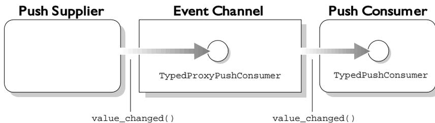
**Figure 6.5:** Transfer of an Event Through an Event Channel to a Consumer Using the Typed Push Model
