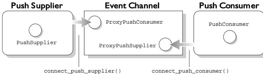
**Figure 6.1:** *Push Supplier and Push Consumer Connecting to an Event Channel in the Untyped Model*
