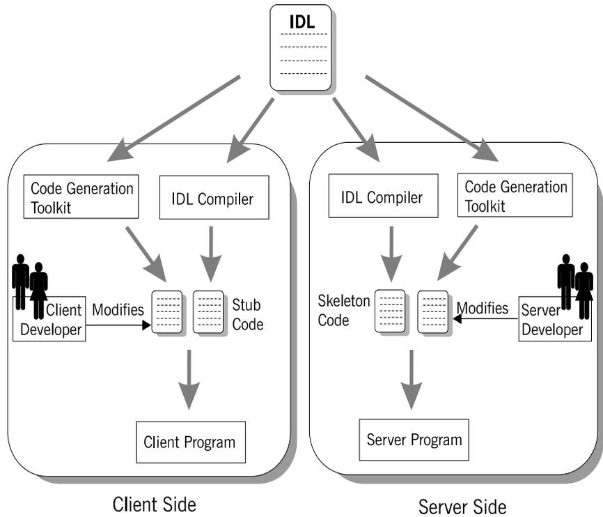
First, you define a set of interfaces written in the OMG interface definition language (IDL). The IDL forms the basis of development for both the client and the server. The toolkit takes the IDL file as input and, based on the declarations in the IDL file, generates a complete, working Orbix application. You can then modify the generated code to add business logic to the application.
