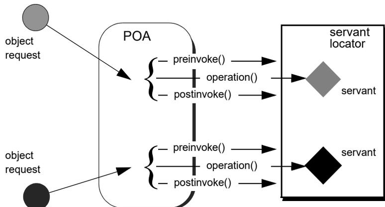
**Figure 17:** The POA directs each object request to the servant locator, which returns a servant to the POA to process the request.
