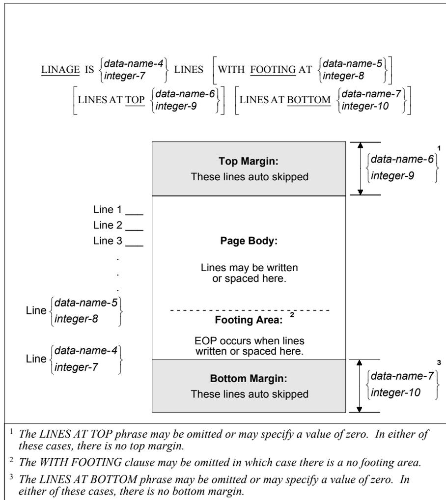
Figure 3 illustrates the logical page layout for a specific LINAGE clause that describes a 66-line logical page.
